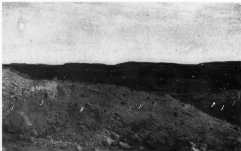
This section of one of the dome-shaped orebodies looks like a porcupine. However, the plugs, not quills, keep the jackhammer holes from being filled up.
